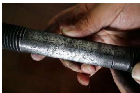
断螺栓呈现纵向裂纹
