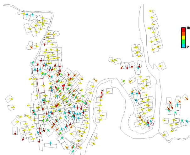
Figure 13 Analysis of the building orientation in Donglei Village
