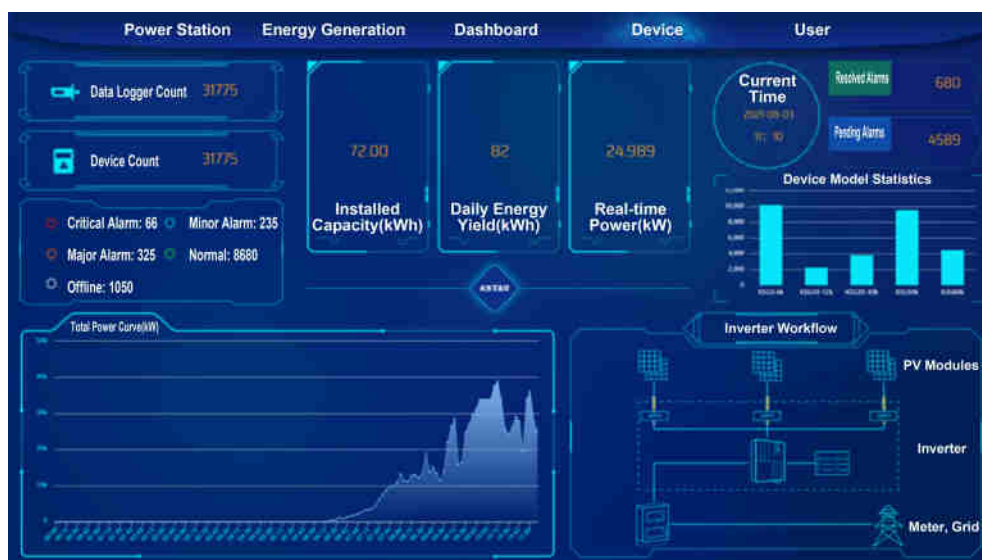
Figure 10 Smart management platform for distributed rooftop photovoltaic systems
