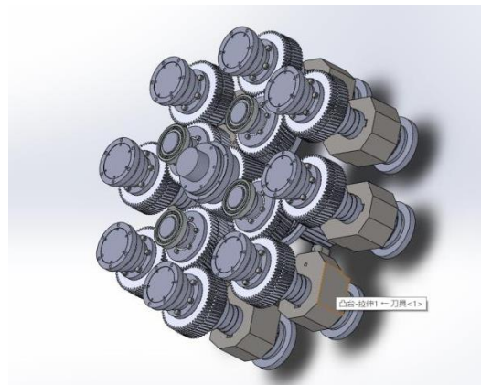
Figure 2 The 3 D model diagram of the boring head
