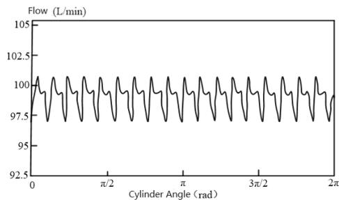
**Figure 11** Flow curve of traditional distribution plate
