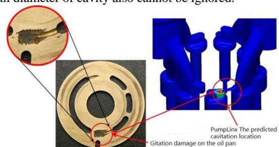
Figure 1 Validation of cavitation on the distribution plate
