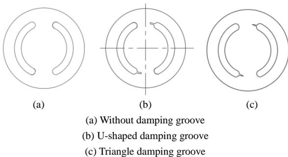
Figure 2 The structure type of the buffer tank
