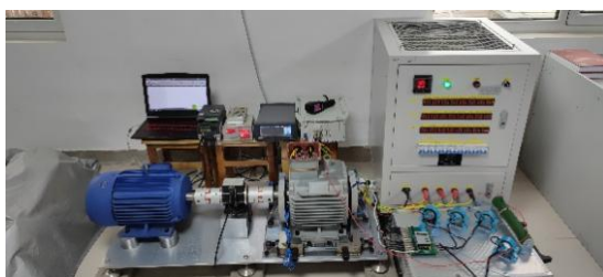
Figure 2 Wind turbine experimental setup
