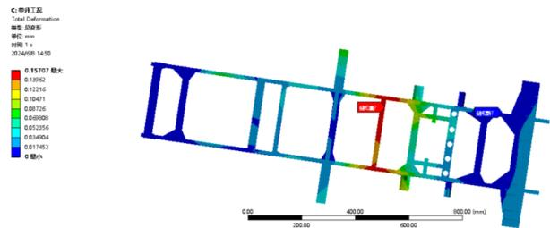
**Figure 11** Deformation diagram of the original frame size under lifting conditions
