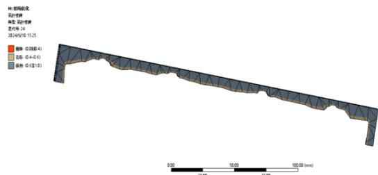
**Figure 16** Optimization results of the second crossbeam
