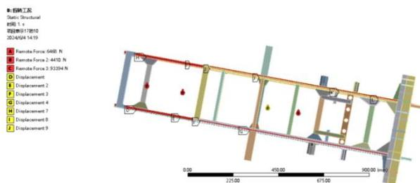
**Figure 6** Load and constraints of the original frame under torsional conditions
