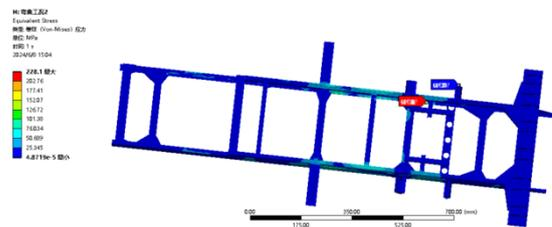
Figure 21 Stress contour of bending condition after optimization
