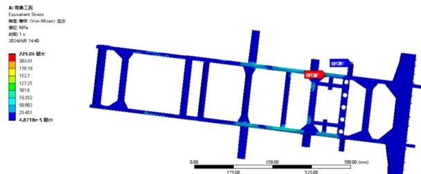
**Figure 5** Stress distribution diagram of the original chassis under bending conditions
