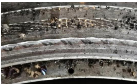
Figure 2 Surface Roughness of the Turned Spigot
