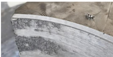
Figure 3 Cutting Texture of the Turned Workpiece Inner Hole
