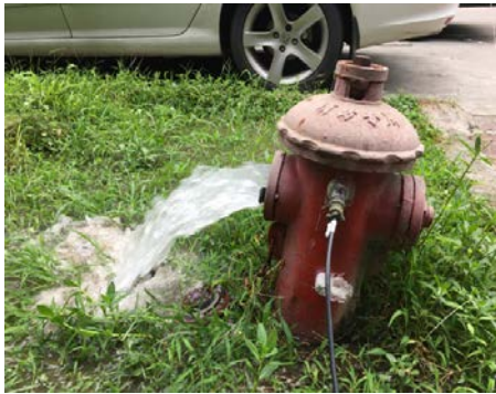
Fig.5 Open fire hydrant to simulate pipe leakage
