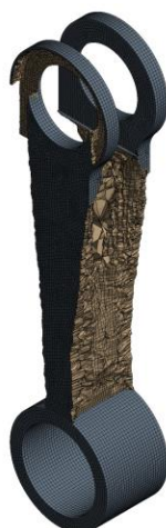
Figure 6 Model comparison before and after big arm optimization
