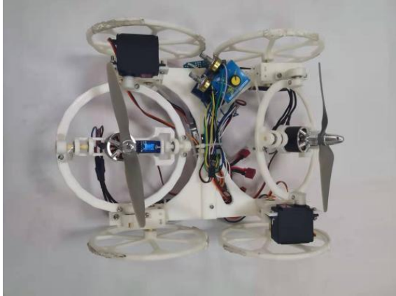
Figure 13 Complete structure of the DHWCR
