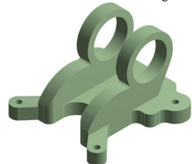
Figure 11 Simplified model after optimization of rotating base
