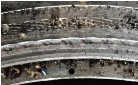
Figure 2 Surface Roughness of the Turned Spigot
