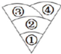
Figure 1 Schematic diagram of V-shaped groove shape
