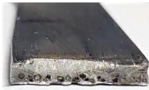
Figure 2 Group of pores on the fracture surface of the unqualified tensile sample (5×)
