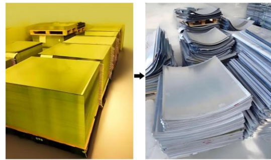
Figure 2 Before and after printing state of aluminum substrate of CTP plates
