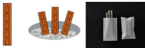
Figure 4 Test method for test bar in freshly mixed concrete
