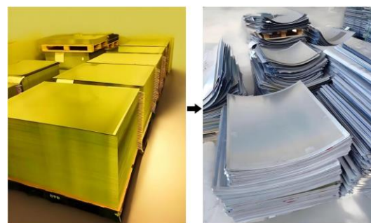
Figure 2 Before and after printing state of aluminum substrate of CTP plates
