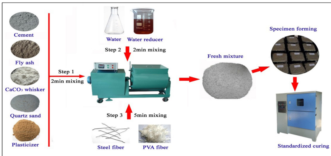
Figure 1 Preparation process of specimens
