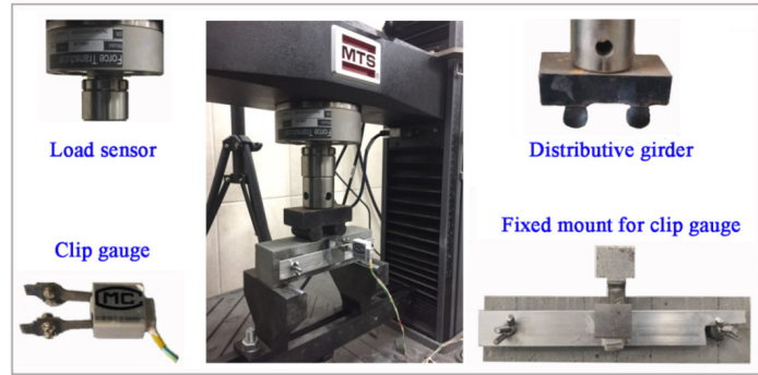
Figure 4 Loading instrument for flexural test
