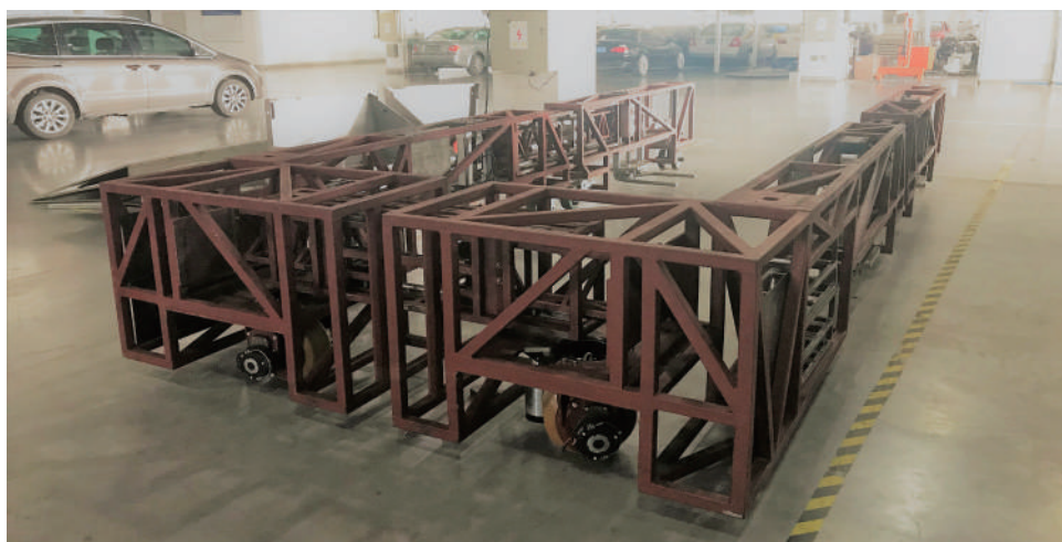
Figure 1. Tongji autonomous parking robot prototype "ITDP-Robot".
