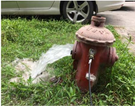
Fig.5 Open fire hydrant to simulate pipe leakage
