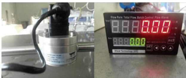
Figure 7 Elliptical gear flow meter for an oil pipeline
