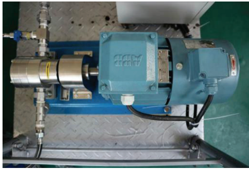
Figure 5 Gear metering pump and variable frequency motor
