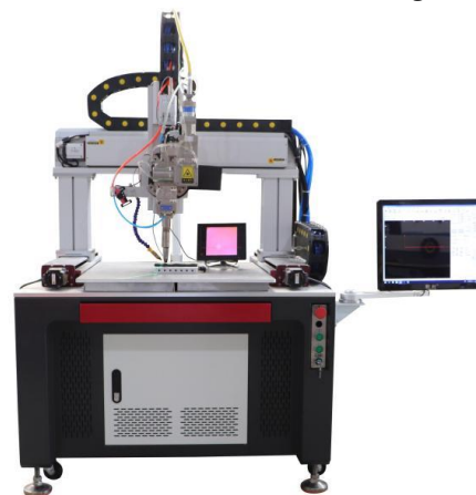
Figure 3 2000W Laser Welding Experimental Platform
