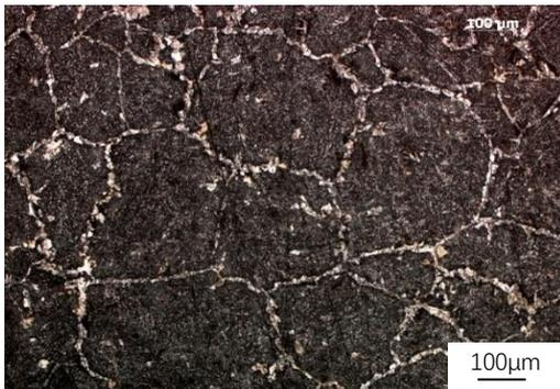
**Figure 2** Ferrite grain size of specimen 0 # X100
