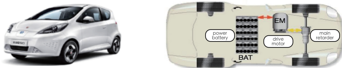
Figure 1 The appearance and powertrain of Roewe E50
